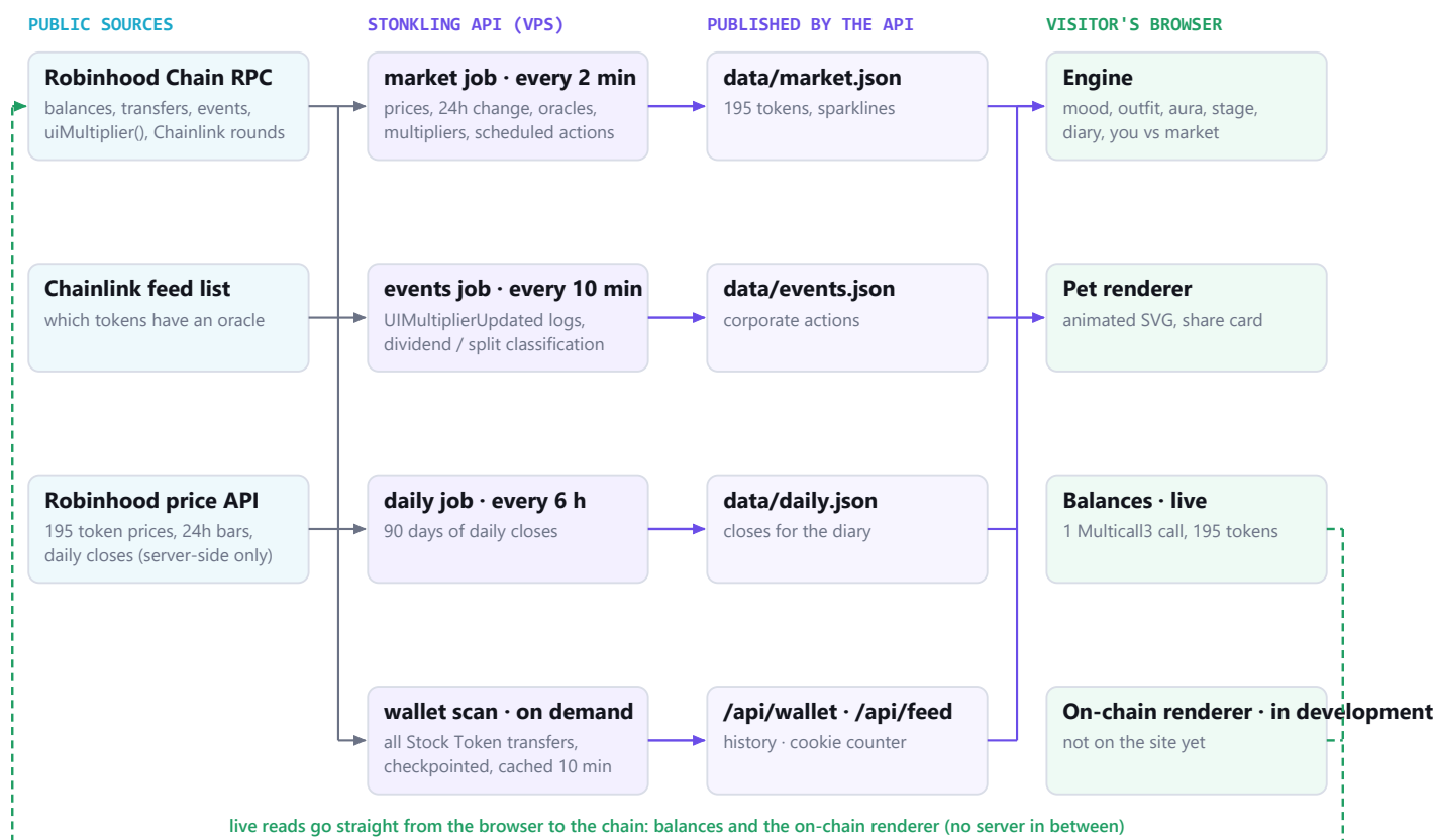
Figure 6. The server only does what a browser cannot (cross-site price data, full-chain wallet scans, caching); balances go straight from the browser to the chain.
